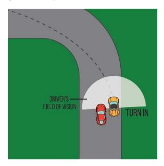
The diagram above shows that the overtaking car has gotten up to the A pillar and into the peripheral view of the lead car before turn in. The overtaking car now has taken the line away and earned the right to racing room on the inside.
