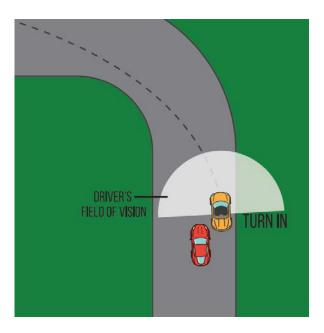
The diagram above shows that at turn in for the lead car the overtaking car has yet to get even with the A pillar and into the peripheral vision of the lead car. The overtaking car is in a blind spot. Do not pass, unless the lead car is much slower and gives racing room.
