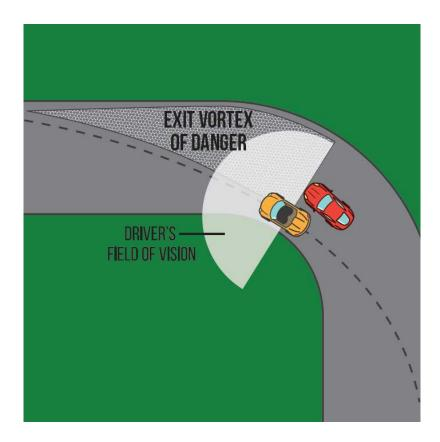
The Exit Vortex of Danger is a triangle inscribed by the apex, the track-out point of the lead car, and the outside edge of the road. When attempting a pass on the outside, be aware of the Exit Vortex of Danger, and back out of it if not in the lead car's vision. It's too late to safely pass. The hole you see on the outside is **closing** rapidly, you are in a blind spot, there will likely be contact, and it will be your fault.
