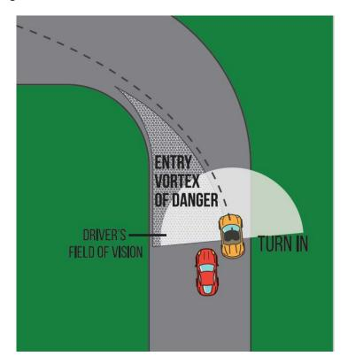
The Entry Vortex of Danger is a triangle inscribed by the turn-in point of the lead car, the apex, and the inside edge of the road. When overtaking, keep out of the Vortex of Danger. It's too late to pass. The hole you see is closing rapidly, you are in a blind spot, there will likely be contact, and it will be your fault.
